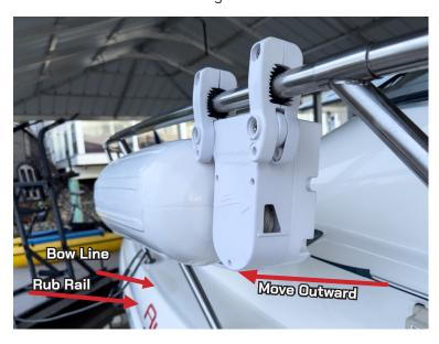
The small hole of the front clamp should be facing out at 45 degrees, the line inserted from the outside.
