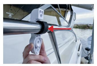
Install the Automatic Fender just in front of the stanchion (towards the Bow). Tighten the bolts only **lightly** to allow clamp movement along the railing during the installation:
