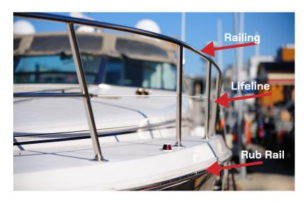
If your cruisers railing is recessed more than 4" relative to the Rub rail, please add the provided spacer. The spacer allows installation closer to the Rub rail by extending the Automatic Fender out from the railing. Add the spacer between the Automatic Fender and the clamp, using the long bolt:
