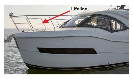
Make sure the lifeline is fully tightened and doesn't interfere with the fender's movement.
