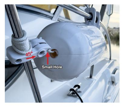
Move the front clamp up or down the Stanchion until the fender is parallel to the railing:
