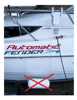
Before docking always confirm that the fenders are deployed to the correct height, and adjust line length if needed.
