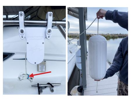
Insert the line from the outside in, towards the Boat, through the front clamp's small hole.
