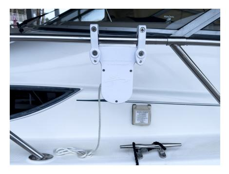
If the Boat has a **lifeline**, it should be placed under or behind the **Automatic Fender**.
