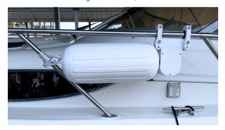
The Automatic Fender line must always wrap over the pulley (from the top), if it wraps from the bottom please refer to troubleshooting:
