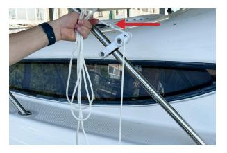
Pull the line firmly while holding the front clamp, and confirm that the knot doesn't slip out through the clamp hole. Wrap the extra line around the stanchion and secure it:
