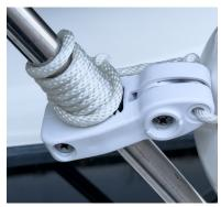
Install remaining Port, and then all Starboard Automatic Fenders in the same manner. In a starboard installation the Automatic Fender is left to the fender, towards the stern. **The Automatic Fender line must always wrap over the pulley (from the top):**
