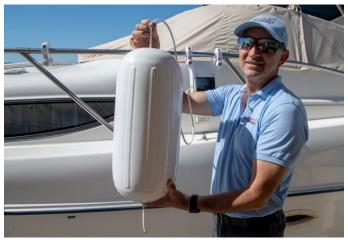
Insert the line from the outside towards the boat, through the front clamp's right hole.
