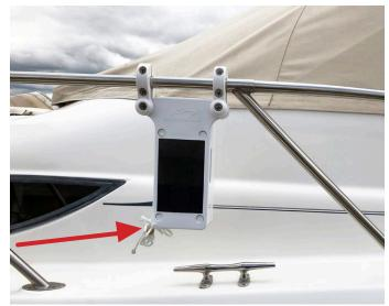
Remove the rubber band from the Power Fender line and run it through the fender's center hole:
