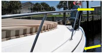
If your cruisers railing is recessed more than 4" relative to the Rub rail, please add the provided spacer. The spacer allows installation closer to the rub rail by extending the Power Fender out from the railing. Add the spacer between the Power Fender and the clamp:
