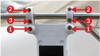
After tightening all lower bolts, tighten all other
