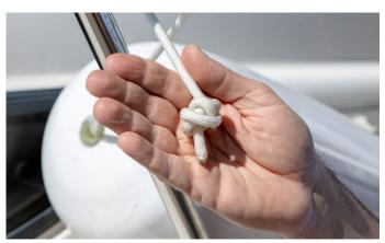
Pull the line firmly while holding the front clamp, and confirm that the knot doesn't slip out through the clamp hole. The first installation stage is complete:
