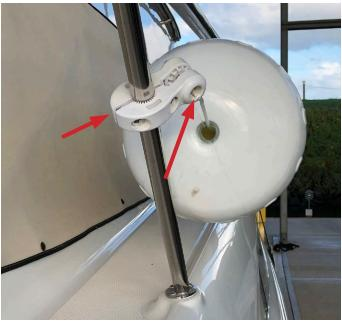
Move the front clamp up or down the Stanchion until the fender is parallel to the railing:
