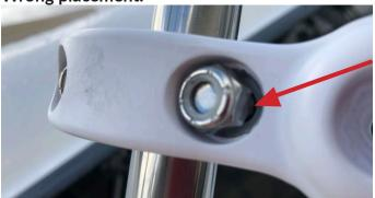
Nut is not fully inserted.
