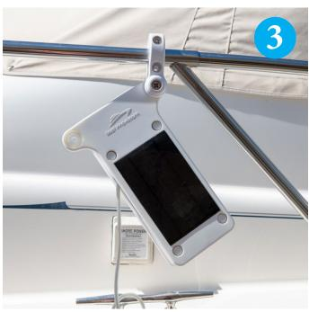
If the boat has a lifeline, it should be placed under or behind the Power Fender. Make sure the lifeline doesn't interfere with the fender's movement. The lifeline should not be too tight, as when temperatures drop it will get tighter and may damage the Power Fender's enclosure.
