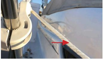
2. Measure your railing height from the water level. For example, if your railing height is 5.5' pull out 6' of line through the front clamp (check following table for your boat's line out). Tie a new knot near the front clamp. Line length to be pulled out:
