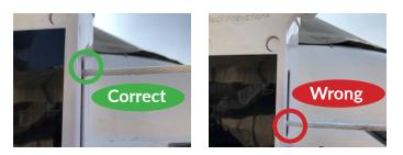
If the fender doesn't go all the way up to the railing, press the switch down and up again. You can always release line by pressing the switch down.
