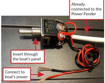
Place the Port switch to the left and the Starboard switch to the right. Connect the power lines to the boat's 12V power only after installing all Port and Starboard Power Fenders and all the fenders on the boat by following all installation steps. Connecting the switch to power before fully installing all Power Fenders may tangle the line and cause a malfunction.
