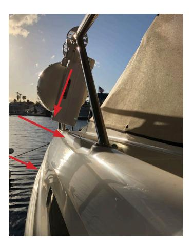
The top of the front clamp should be facing out at 45°, the line inserted from the outside.
